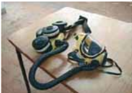
Example of full-face vapour mask with belt-mounted filter unit
