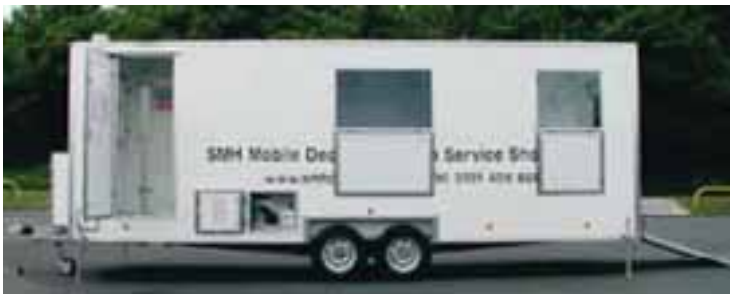
FIGURE J5 Example of trailer-mounted, three-stage decon unit 3
